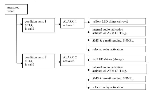
Example of alarm creation at used logical combination of conditions:
