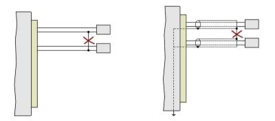
• **do not create hidden earth loops** - do not connect cable shielding at end device side, if these device do not have terminal designed for shielding. Shielding must not be connected to outer metal parts of the device nor with other devices. Do not use shielding as a signal lead.
