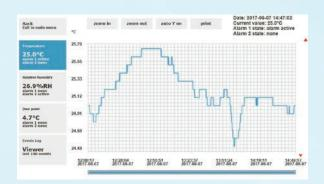
**Graphs of current values** can be accessed via a web browser, offering the capability to display up to one thousand measured values per channel.
